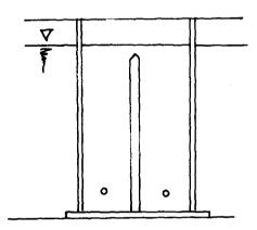
(1) The day's rainfall has exceeded the evaporation and the tip of the fixed point gauge is submerged.
