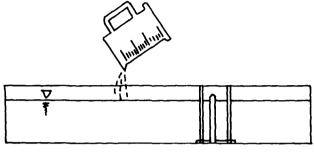
(3) The water is poured into the evaporation pan, raising the water level by 2.0 mm., but the point gauge is still exposed.
