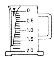
(5) The measuring can is filled a third time up to the zero level
