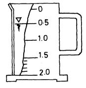
(6) At this time the water level reading in the measuring can is 0.5 mm. which means that 1.5 mm. of water has been removed from the evaporation pan.
