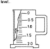
(8) At this time the water level reading in the measuring can is 1.2mm
