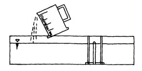
(6) The contents of the measuring can are added slowly to the pan while carefully noting the water level relative to the point gauge.
