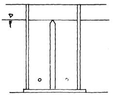
(7) The water level in the point gauge cylinder is at the tip.
