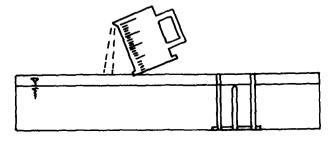
(5) The contents of the can are added slowly back into the pan while carefully noting the water level rising up to the exact tip of the point gauge.
