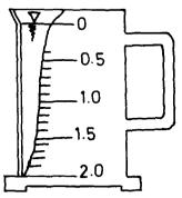
(3) The can must be filled only to the zero level and not to the very top of the can. Empty the can.
